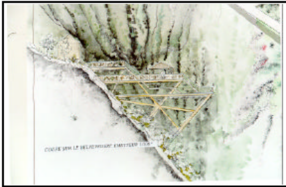
An architectural lookout could hide the projecting array under its supporting structure as an alternate solution to landscape integration
